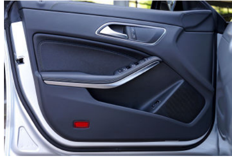
Photo 14 Driver's door trim panel.
